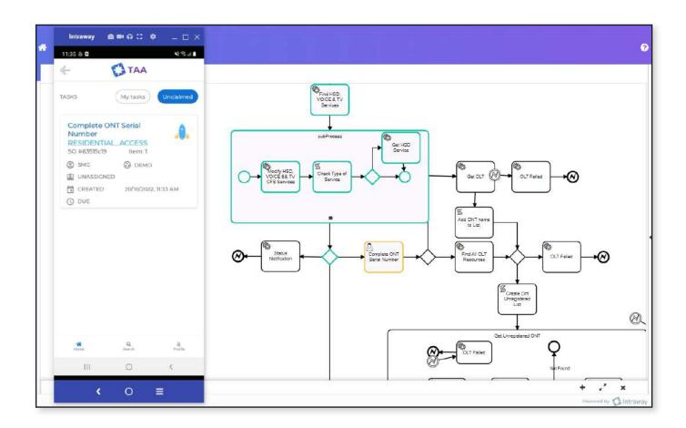
Using the Intraway <u>Tech Assist App</u>, a technician can claim a task or tasks related to provisioning this Ethernet service. Several components or domains need to be configured:
